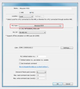
**Step 3.** Change the driver back to Mitsubishi FX3U/FX3G. Now "Interval of block back", "Max. read-command size" and "Max. write-command size" are updated to 5, 32, 32.
