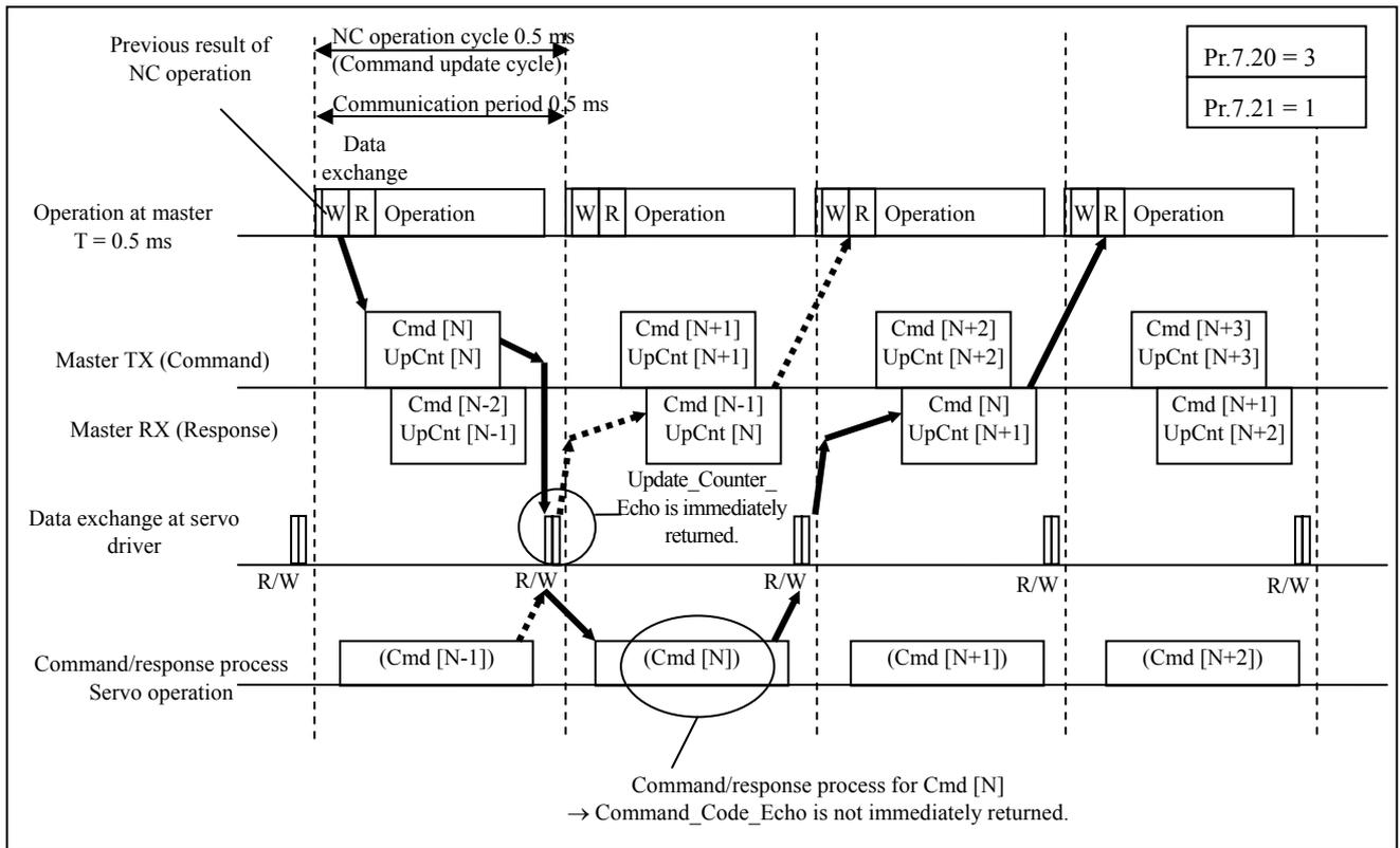
3-1-2 Transmission timing of communication cycle 0.5 ms/command updating cycle 1.0 ms
