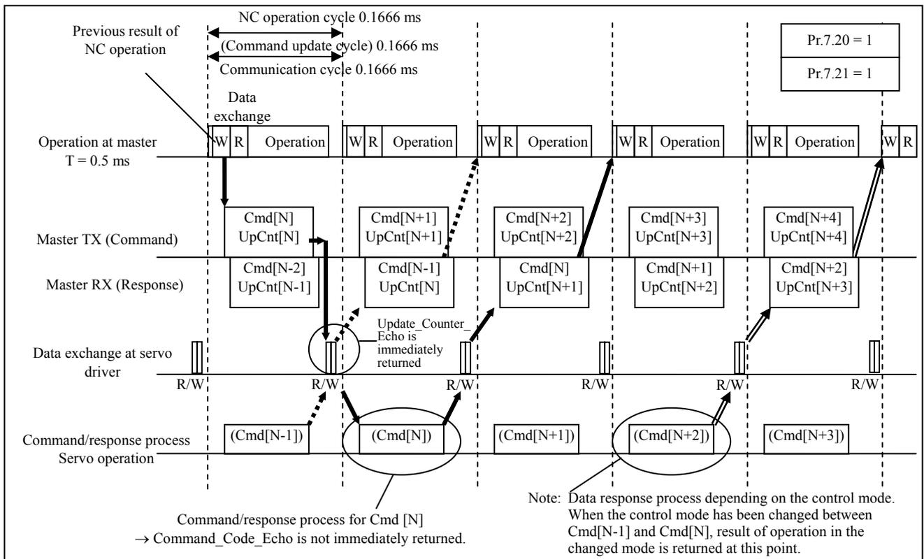
3-1-4 Transmission timing of communication cycle 0.0833 ms/command updating cycle 0.1666 ms
