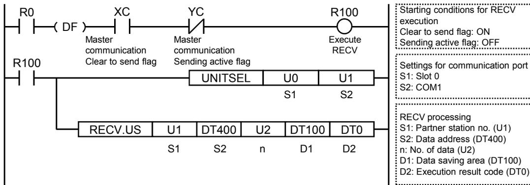
(Note) The unit number and COM port number in the above program is applied when the COM.1 port of the CPU unit is used.
