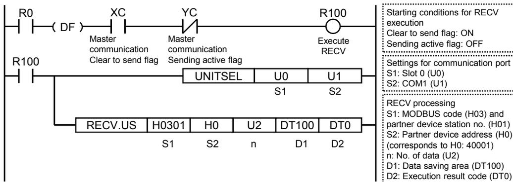
(Note 1) Operand [S1] of RECV instruction is specified by combining two hexadecimal digits of MODBUS function code with two hexadecimal digits of partner device station no.
