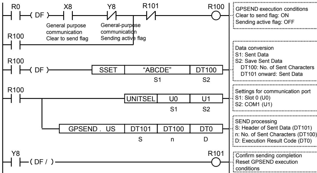
(Note) The unit number and COM port number in the above program is applied when the COM.1 port of the CPU unit is used.
