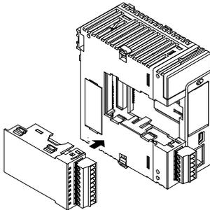
The illustration is the CPU unit. As for the Serial Communication Unit, the attachment procedure is the same.
