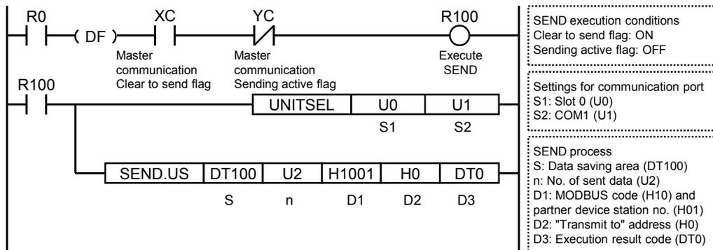
(Note 1) Operand [S1] of SEND instruction is specified by combining two hexadecimal digits of MODBUS function code with two hexadecimal digits of partner device station no. When the MODBUS function code is 16, specify H10 for [D1].
