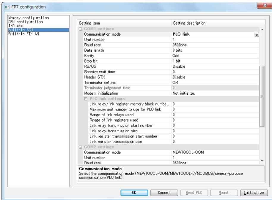
**4. Specify conditions to be allocated to each setting item for "Station no." and "PLC link settings" under "COM1 settings", and press [OK] button.**
