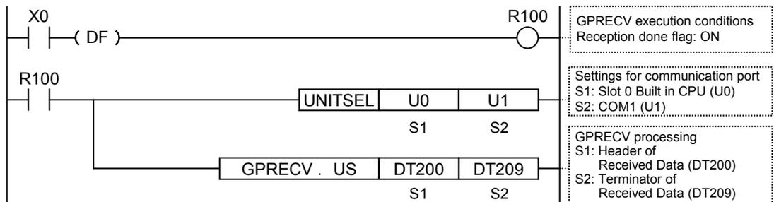
(Note) The unit number and COM port number in the above program is applied when the COM.1 port of the CPU unit is used.
