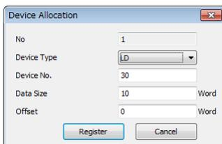
In this example, "Device Type = LD", "Device No. = 30" and "Data Size = 10".
