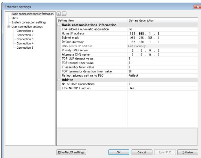
2. As necessary, change "Home IP address" and "No. of User Connections".
