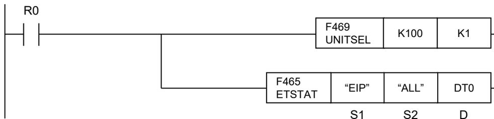
(Note 1): The figure above shows the case of specifying a communication unit slot number (Ethernet communication = K100) using F469 UNITSEL instruction.
