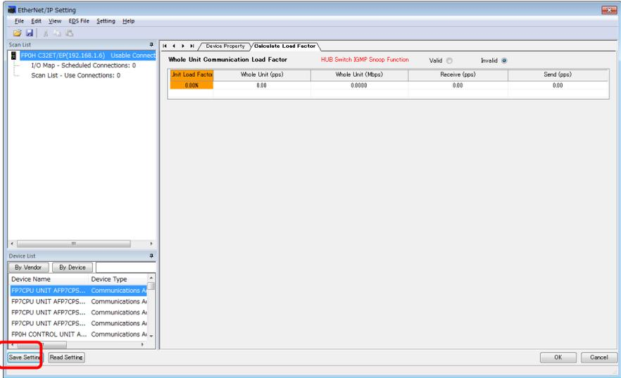
1. **Press [Save Settings] on the lower left of the EtherNet/IP Setting screen.**
