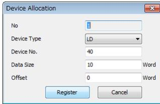
In this example, "Device Type = LD", "Device No. = 40" and "Data Size = 10".
