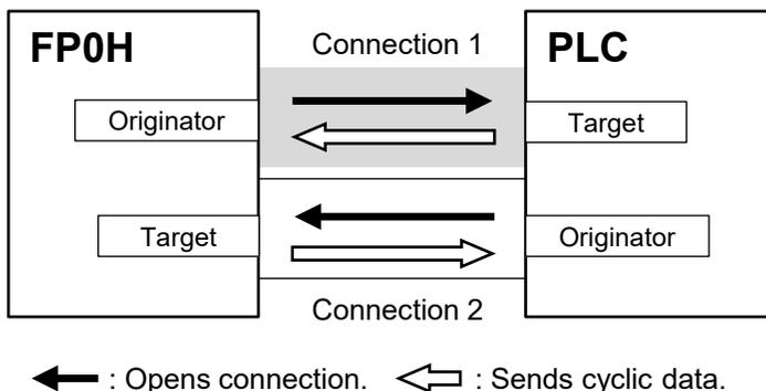
For the communication between the FP0H and other I/O devices, the FP0H is the originator. According to devices, the data transmissions by "Input Only" (from target to originator) and "Exclusive Owner" (two-way) may be available.
