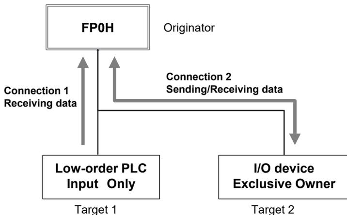
Register target low-order PLCs and I/O devices in "Scan List" of FP0H and register connection information. The registration is made for each target.
