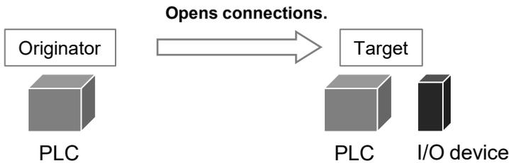
Connection information on the cyclic communication is set in the originator. The originator connects to the target according to the connection information. The tag/instance required for the connection from the originator is registered in the target.
