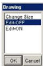
Here is the drawing dialog (see p. 129) when you have defined the method direct, for example, with number of replacements = 10. The custom part will assume 1 of 10 appearances based on which reference device is active.
