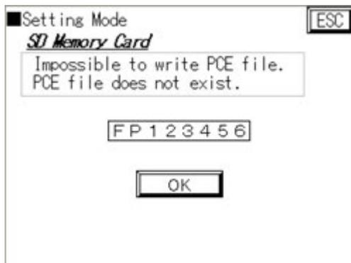
In this case, check the contents of the SD memory card. Either the PCE file has the wrong file name (it must be the same as the corresponding FP file) or it has not been created yet. If the PCE file has not been created yet, start FPWIN Pro and create the FP and PCE file with the commands listed above.
