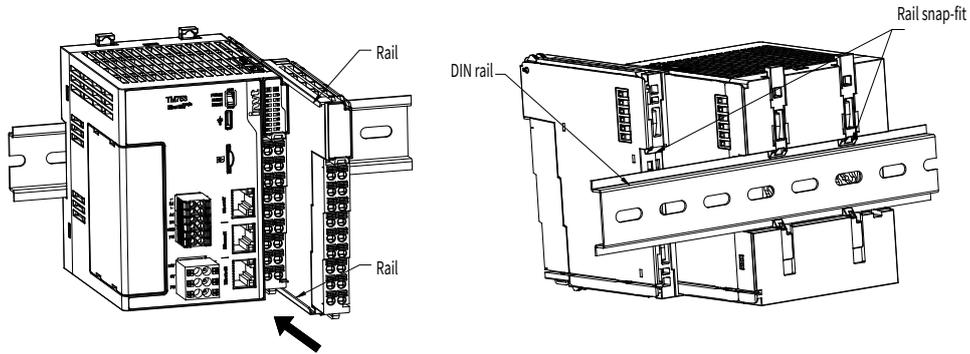
**Note:** The master and the module use DIN rail for installation.
