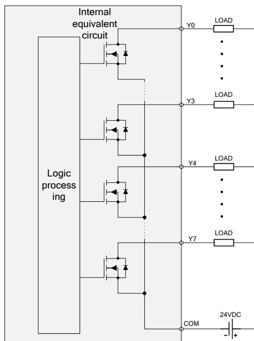
**Note:** The flyback diode is needed for external inductive load connection. The wiring diagram is shown as below.
