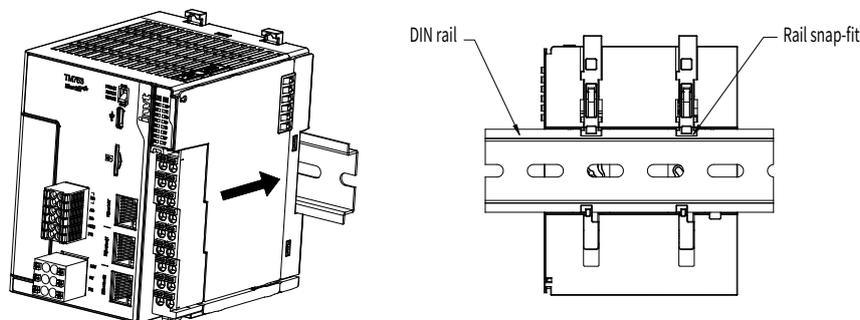
**Note:** The master uses DIN rail for installation.
